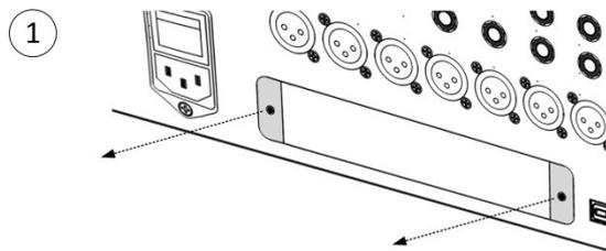
Align the uTrack-X32 option card with the card guides, then push it all the way into the internal connector socket.
